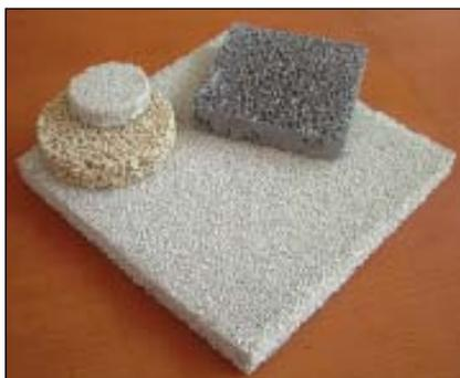
Examples of ceramic foam filters, which can be quickly dried without warping.
